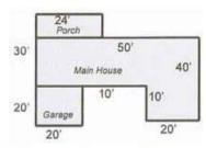
Imagine that this house has a single brick foundation wall, concrete driveway, concrete attached slab, and 18 16"x8" block piers.
